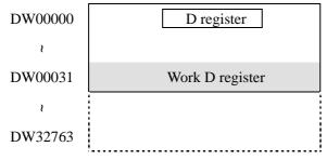
Work D register allotted from the following addresses of D register number which the user set, and prevented D register which the user used with the ladder in the program and the address the overlap.
